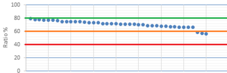
Graph 2 – Distribution of VSC ratio reductions of window that failed VSC test
